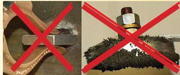
Stays clean. Turn off Magswitch and wipe away debris.
