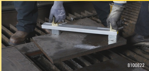
Pivot handle allows use as a hand lifter or a sheet dragger. 8100359
