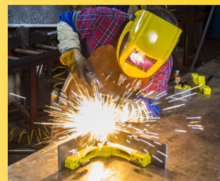
Each magnet holds on two sides.
