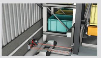
No interference between the DDLS 500 and AMS 300i distance measurement system
