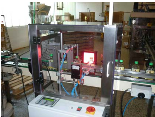
Figures 4a and 4b. With the rear-illumination method, the fill level is visible as a dark line – emphasized by the refraction at the liquid surface.
