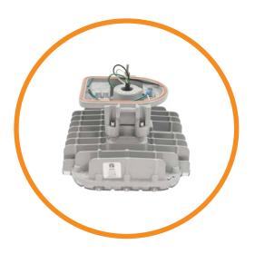
Dialight's innovative Universal Mounting Adapter (UMA) simplifies installation to save time and money while improving safety. Our integrated hinge-style bracket system comes pre-installed, allowing installers to simply mount the bracket to the wall, ceiling or stanchion, where it hangs safely in place while the installer makes electrical connections. After installation, the sealed wiring compartment protects those connections against dust and moisture ingress.
