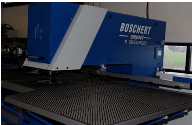
Figures 4a, b. Boschert Compact punching machine ...
