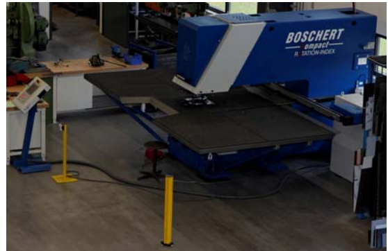
... and in practice. At the front clearly recognizable: The UMC deflecting mirror columns for access guarding on several sides
