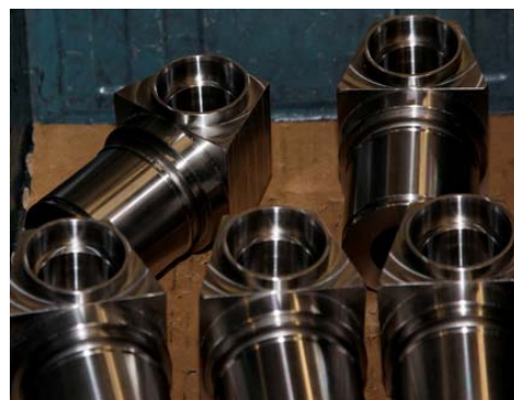
Figures 2a, b, c, d. A wide variety of work pieces made from metal: Formed plate, lathed and milled parts
